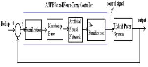
Figure-7 Block diagram of ANFIS based Neuro-Fuzzy Controller
