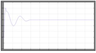
Fig-9(b) Change in wind power generation for the step load change of 2%(0.02p.u.)
