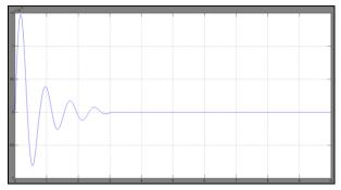
Fig-9(a): Frequency deviation of the hybrid system for the step load change of 2%(0.02p.u.)
