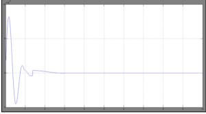
Fig-10(c) Change in diesel power generation for the step load change of 4%(0.04p.u.)
