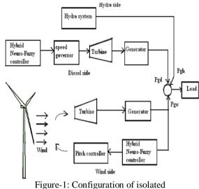
wind - micro hydro diesel hybrid system
