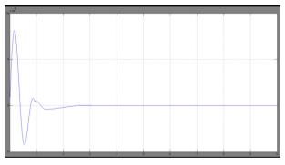
Fig-9(c) Change in diesel power generation for the step load change of 2%(0.02p.u.)
