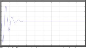
Fig-10(d) Change in hydro power generation for the step load change of 4%(0.04p.u.)
