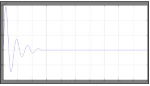
Fig-10(a) Change in frequency for the step load change of 4%(0.04p.u.)
