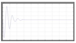
Fig-9(d) Change in hydro power generation for the step load change of 2%(0.02p.u.)
